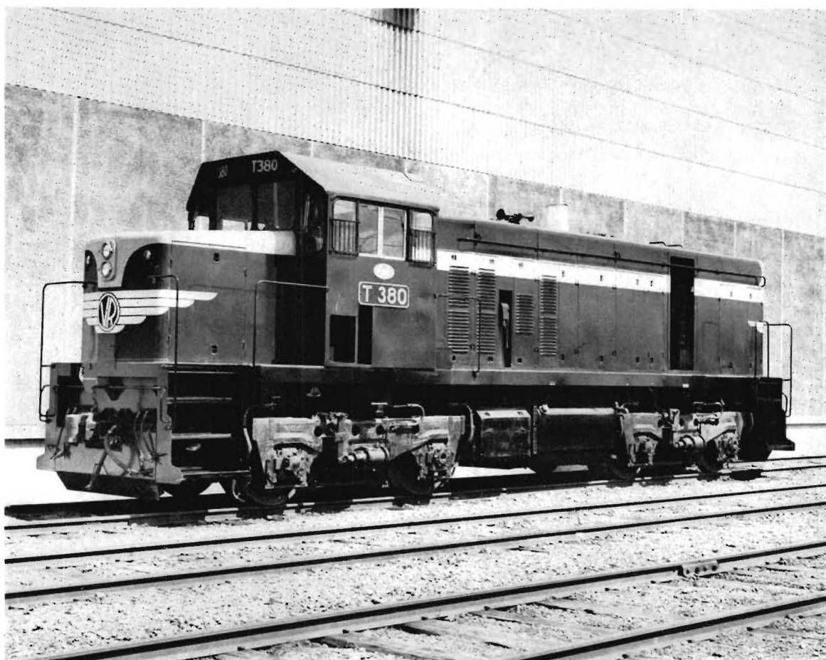
'T' Class 950 h.p. Diesel-electric Locomotive.
